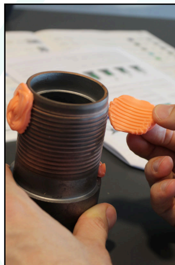
P35 external form cut with the Double Blade Cutter
