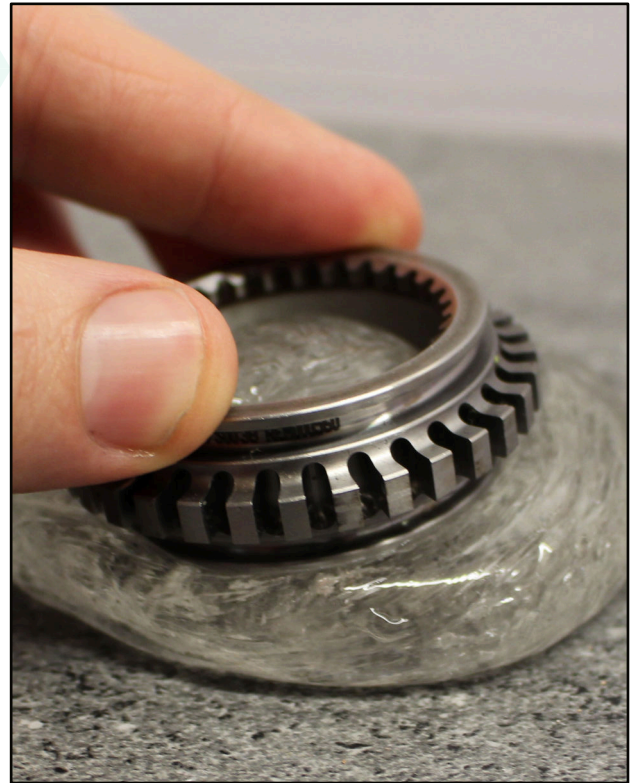
Re-FORM (in its hot, soft state) receiving a part to be held in place.
